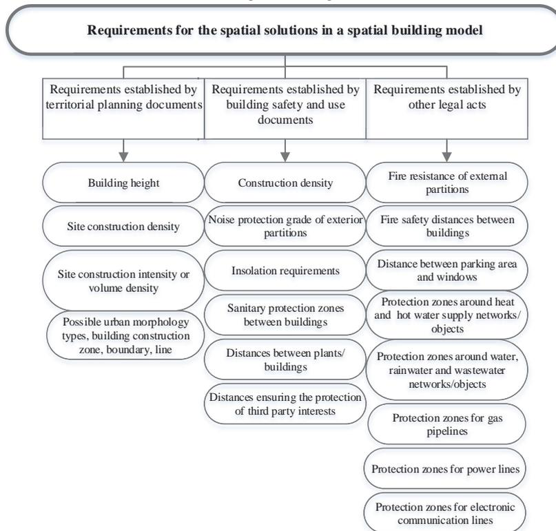
Fig. 4. Requirements for the spatial solutions in a spatial building model.
