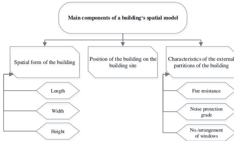
Fig. 3. Main components of a building's spatial model.
